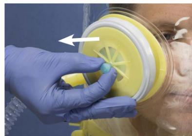
**15.** Fit the access port cap then pull the anti-asphyxiation button until the hood inflates.
