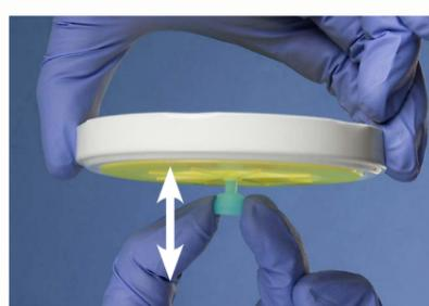
**5.** Check the smooth operation of the bi-directional anti-asphyxiation valve and place to one side.
